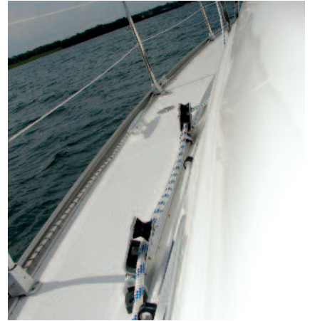
The placement of the Genoa tracks tight to the cabin top allow easy forward movement.
